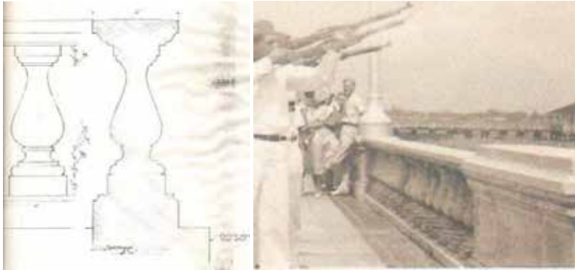
Above, original design detail of balustrade (courtesy Olmsted NHS) and circa 1949 appearance (courtesy JHS); below, current profile with added cap layer. Note also exposed, rusting reinforcing steel.
